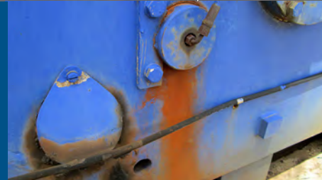
Fig. 10 — Rust comes from one of the trunion wheel bearings of this gantry crane above. There was no sign of corrosion prior to the salt water inundation from Hurricane Sandy.
