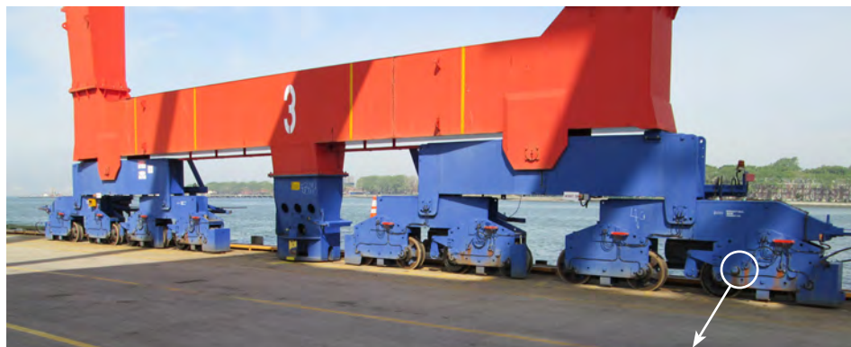
Fig. 10 — Rust comes from one of the trunion wheel bearings of this gantry crane above. There was no sign of corrosion prior to the salt water inundation from Hurricane Sandy.
